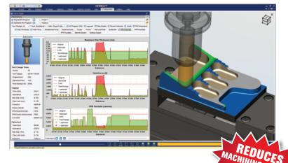
ties. Based on the cutting tool geometry, part material, and programmed cutting conditions, VERICUT automatically determines the optimum safe feed rate for each cut. The VERICUT optimized NC program will greatly improve cutter performance resulting in significant cycle time savings, reduced tool wear, improved tool life, and better finished parts.
